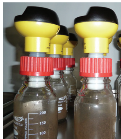
OxiTop® system for short term respiration test, Niefern, Germany
