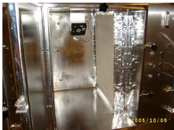
Fig. 1. Insulation material in full construction in test chamber.
