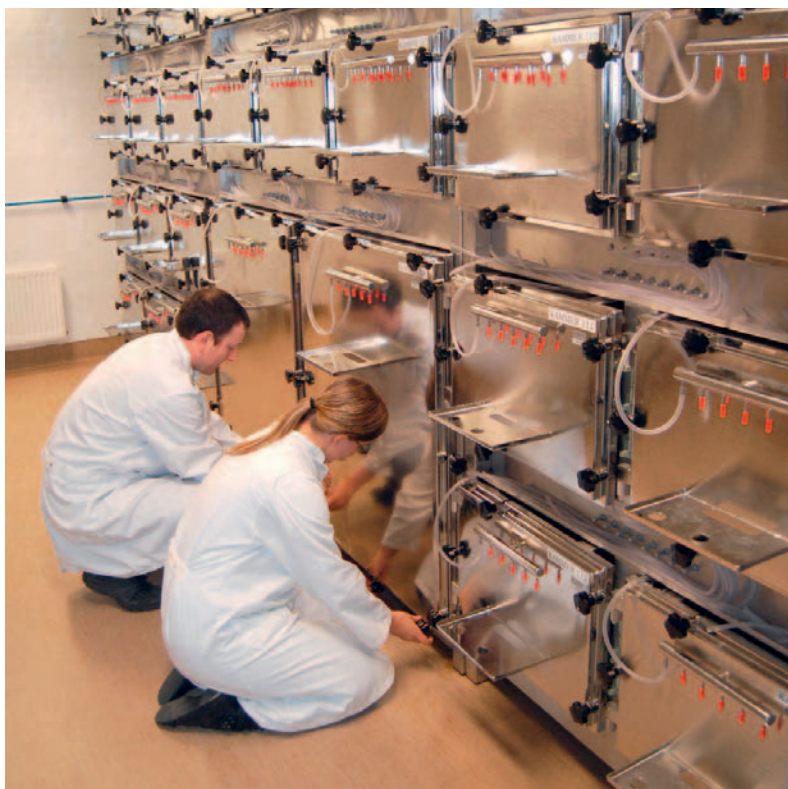
Figure 2: Ventilated emissions test chambers are made of stainless steel
