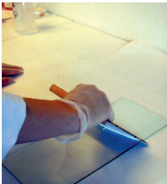
Figure 1: Application of an adhesive onto glass for emissions testing
