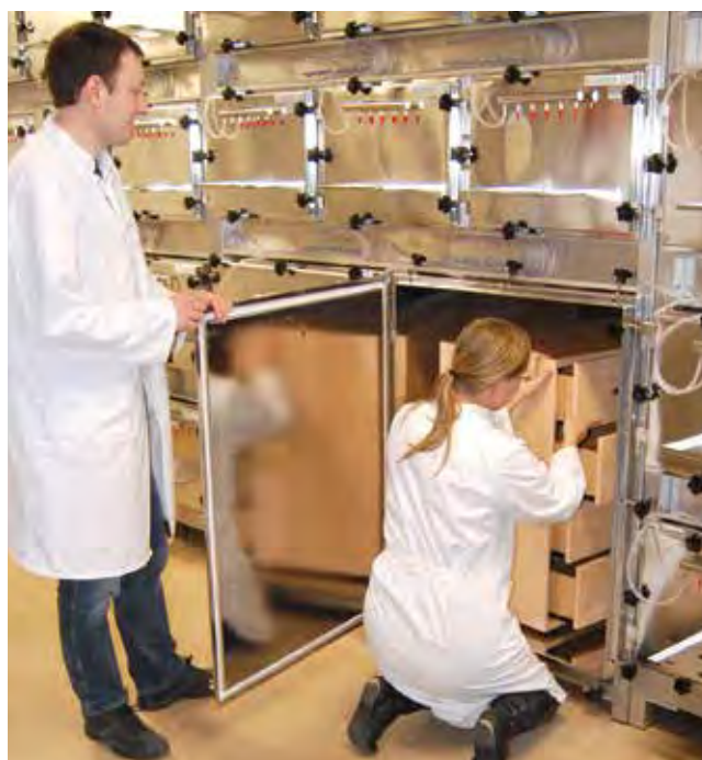
For a non-uniform test specimen such as furniture, Eurofins performs full object testing in large chambers.
