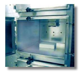
French AFSSET agency published the "Protocole AFFSET" guideline for limiting VOC emissions into indoor air. It specifies chamber emission testing and limit values after 3 and after 28 days of storage in a ventilated test chamber - the 28 days test is regarded as representative for long-term emissions. The test method is ISO 16000 (parts 3, 6, 9, 10 and 11), and the results are calculated to the European reference room of 3 m x 4 m x 2.5 m with ½ air change per hour.
